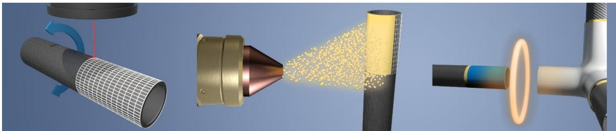
*Figure 1: Process chain consisting of laser pre-treatment of CFRP, thermal spray deposition of a copper coating, low-temperature soldering to a steel counterpart to produce a three-dimensional multi-material joint; © Fraunhofer IWS*
