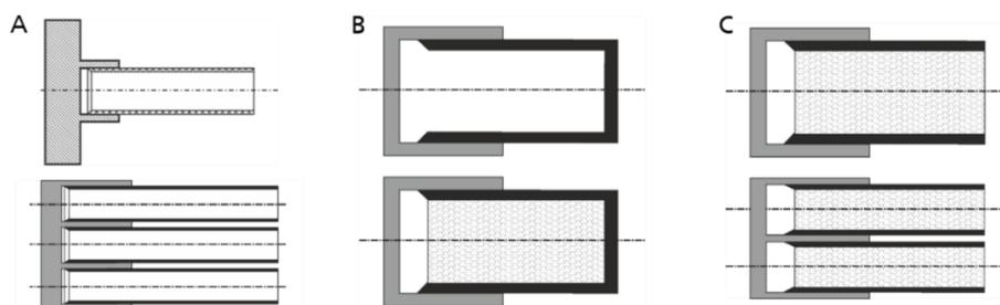
Figure 2: FRP tubes as crash elements, tubes arranged in several rows (A); FRP C-profile, foam core stabilizes walls during crash (B); Sandwich with FRP cover layers and foam core, foam core stabilizes cover layers during crash (C) [5]
