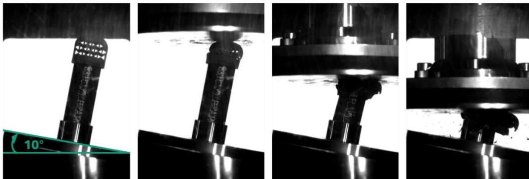
*Figure 3: High-speed oblique test (8.9 m/s) with CFRP crash tube and auxetic force introduction element*
