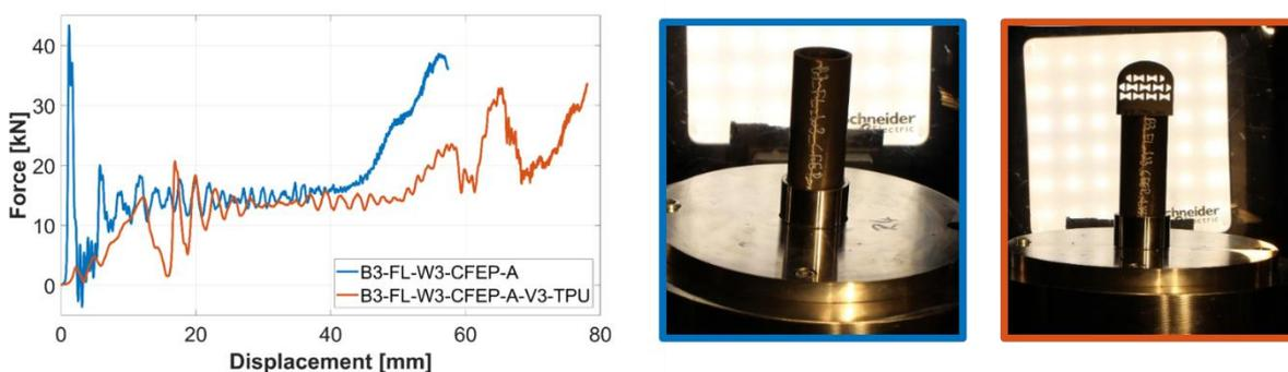
*Figure 4: Influence of the auxetic force introduction element on the force-displacement curves*
