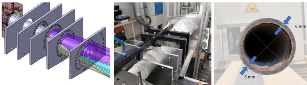
*Figure 12: Pultrusion in the preparation, guiding panels, pultruded profile (left to right)*
