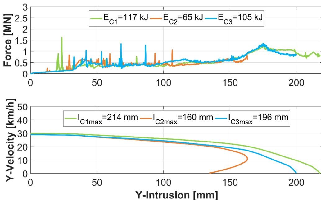
Figure 9: Numerical results: force-displacement diagram with the absorbed Energy values (top), velocity-displacement diagram with the max. intrusion values in global Y-direction (bottom); LS-DYNA solver version: R10.1, with the preset: message passing parallel (mpp\_d\_R101)
