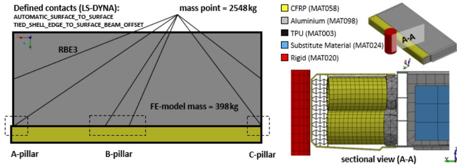
Figure 7: Considered geometry, mass, and material models in the simulation
