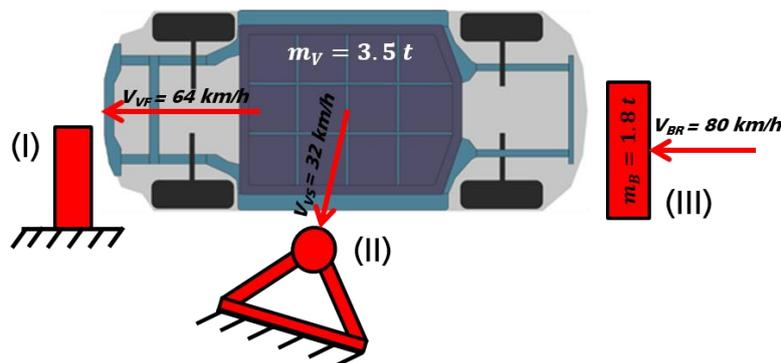
Figure 1: Load cases to be considered for the development of a crash protection for the vehicle platform
