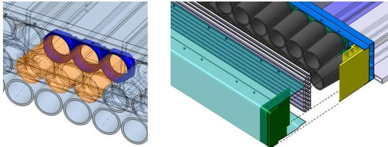
Figure 10: Left: crash tube mount, right: auxetic buffer element (grey), detachable two part node (green, yellow)
