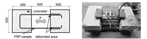
Figure 4: Determination of the stirrup tensile strength according to ACI Committee 440 Method B5 (left: test setup, right: hydraulic cross beam with sensors)
