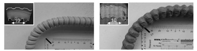
Figure 2: Sample of FRP stirrup (left: GFRP cladding tube, right: GFRP winding)
