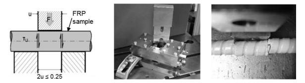
Figure 5: Determination of shear strength according to ACI Method B4 (left: diagramme, centre: device, right: specimen after testing)
