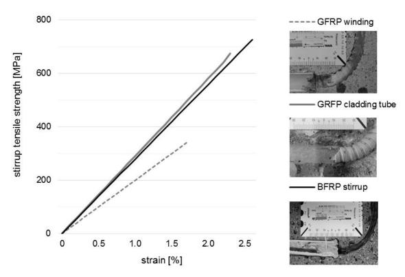
Figure 7: Tensile strengths in the curve area
