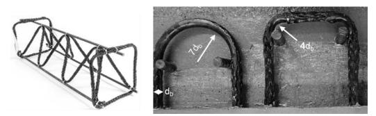
Figure 9: Comparison of FKV reinforcement with large and small radii of curvature
