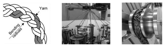
Figure 3: Production (left: principle, centre: semi-finish production, right: forming process)
