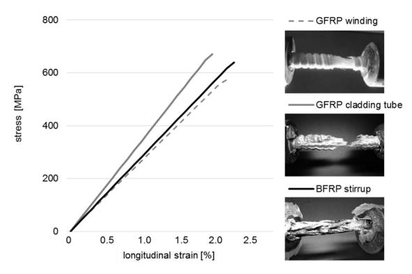
Figure 6: Uniaxial tensile test
