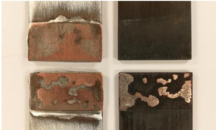
Figure 7: Fracture surfaces of two wire arc-sprayed copper coatings on CFRP with different surface pre-treatments (top: laser roughening, bottom: R+TS) soldered to a steel sheet
