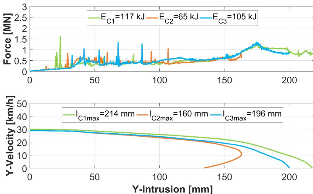
Figure 9: Numerical results: force-displacement diagram with the absorbed Energy values (top), velocity-displacement diagram with the max. intrusion values in global Y-direction (bottom); LS-DYNA solver version: R10.1, with the preset: message passing parallel (mpp\_d\_R101)
