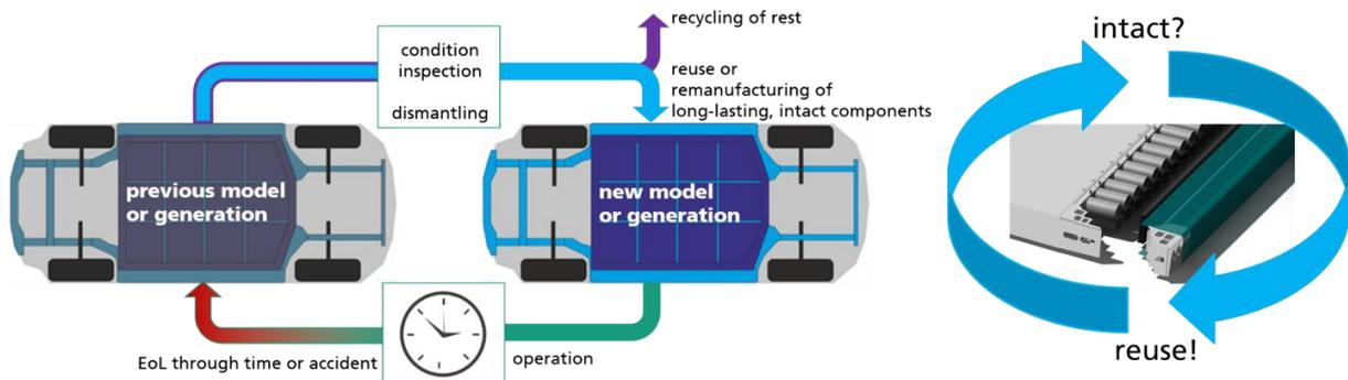
Figure 6: Schematic reuse and cycling representation of long-lasting, intact components for sustainable mobility
