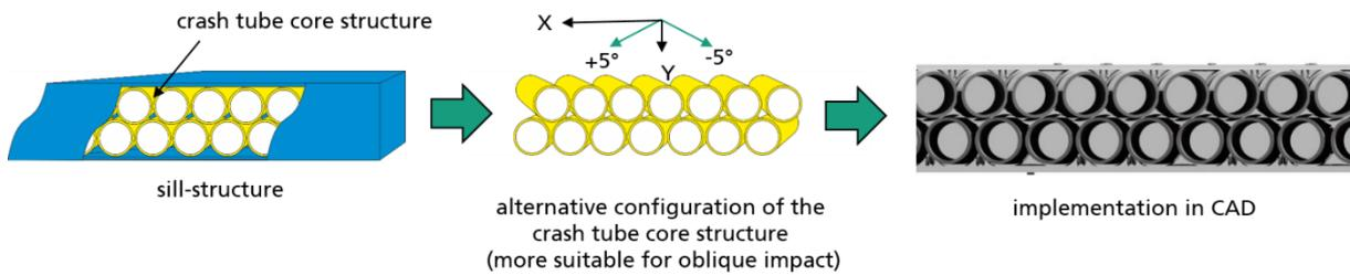
Figure 5: Concept for the alignment of the crash tubes in the sill structure
