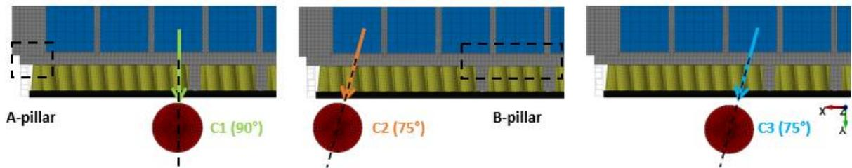
Figure 8: Defined load cases based on EURO NCAP
