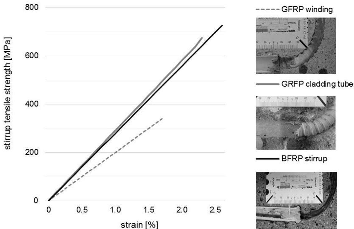
Figure 7: Tensile strengths in the curve area
