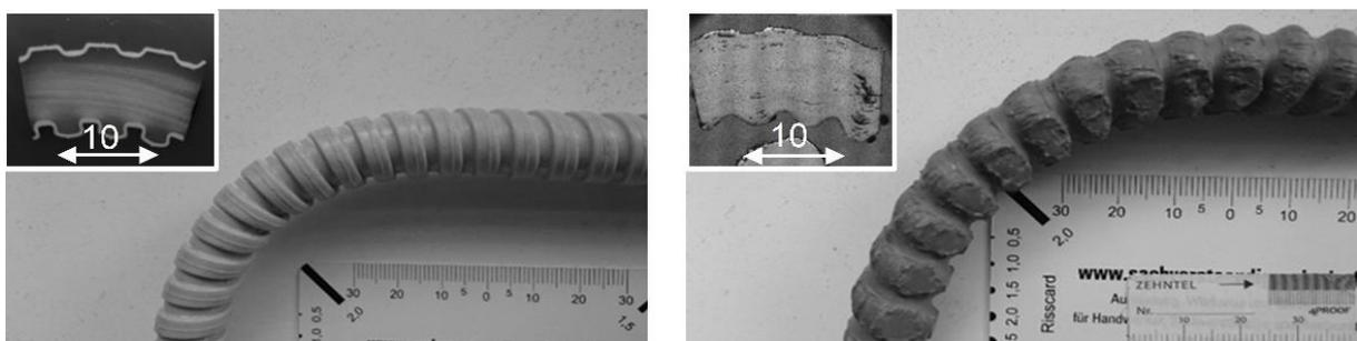
Figure 2: Sample of FRP stirrup (left: GFRP cladding tube, right: GFRP winding)
