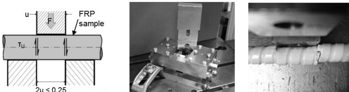
Figure 5: Determination of shear strength according to ACI Method B4 (left: diagramme, centre: device, right: specimen after testing)
