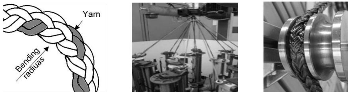
Figure 3: Production (left: principle, centre: semi-finish production, right: forming process)
