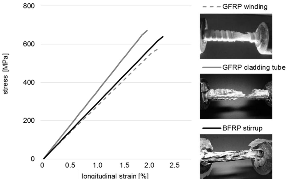
Figure 6: Uniaxial tensile test
